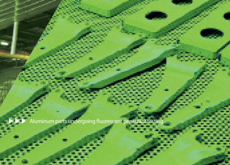
▶▶▶ Aluminum parts undergoing fluorescent penetrant testing
